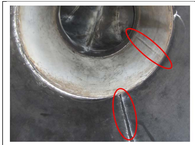
Example image for the orientation of the manufacturing weld seams of the piping after assembly
