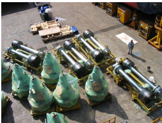
Main pistons and cylinder covers (still covered and exhaust cage closed by plate)
