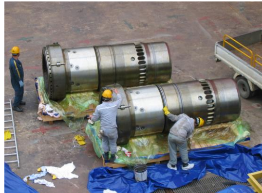
Cylinder liners at cleaning stage at shipyard.
