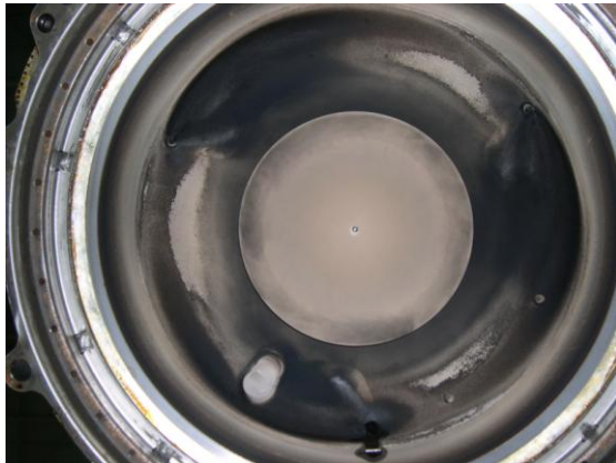
Combustion chamber with carbon deposit after shop test.
