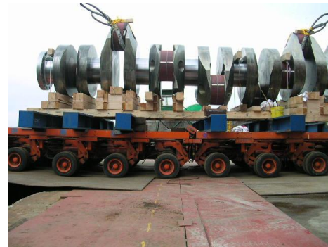
Crankshaft delivered as single part. Already cleaned of corrosion protector by solvent and ready for bedplate assembling. Crank-throw journals protected with rubber and steel plates (8mm thick).
