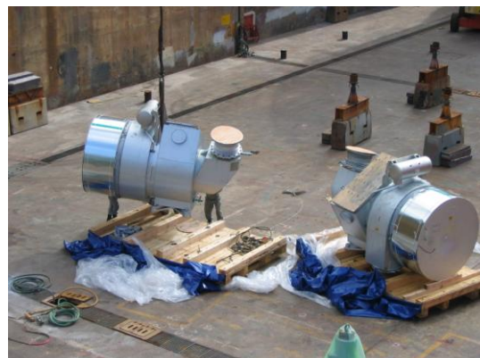
Turbocharger prepared ( openings closed by wooden plates)
