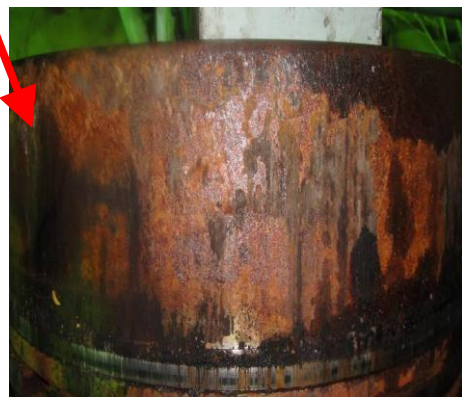
Heavily corroded: Cylinder liner and piston crown. At last the parts could be pulled or reached to be cleaned and judged for further procedure (replacement).
