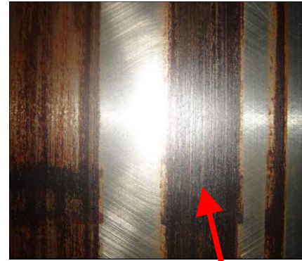
Repaired (cleaned of upper rust layer) cylinder liner (above) and piston crown (below) surface revealed that the pitting had been so heavy that the parts had to be replaced.
