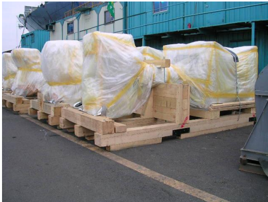
Example of connecting rod with crosshead at transport packaging stage. Stored outside just after arrival at shipyard.
