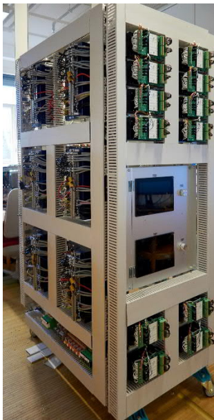
Figure 16. Hardware-in-the-Loop (HIL) test rig. Visible are the CCUs, left side, and two MCPs and several load cards for actuators on the right-front side.
