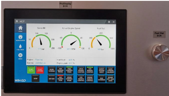
Figure 9: WiCE – Manual Control Panel (MCP) with touch screen and fuel dial.
