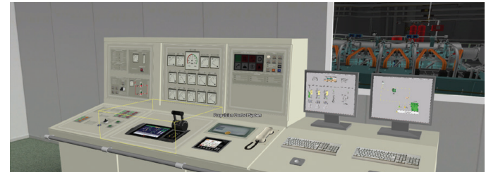
Example of an action screen: Engine Control Room with zoom-in on the interface of the Propulsion Control System
