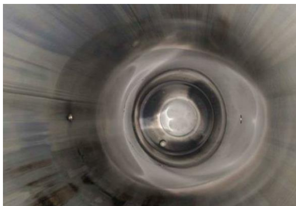
Figure 3 – cylinder liner of a X62DF engine in excellent condition (with visible gas nozzles in mid stroke position).
