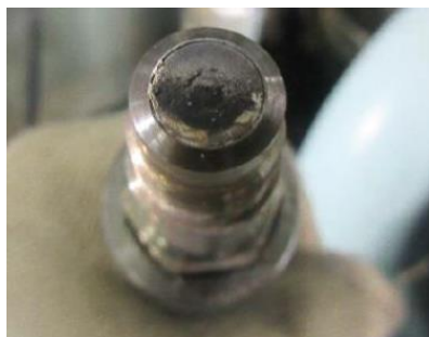
Figure 1 – Cylinder pressure sensor with surface deposits
