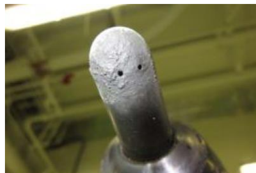
Figure 2 – Fuel injector nozzle tip with 3 (out of 5) clogged atomizer spray holes
