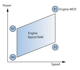
Any power and speed within the respective engine layout field may be selected as the Contracted-MCR (CMCR) point for an engine.
