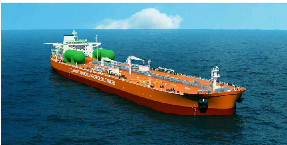
A 3D model of two of the world's first ammonia dual-fuel Aframaxes to be constructed with six-cylinder X62DF-A engines by Dalian Shipbuilding and owned by AET.
